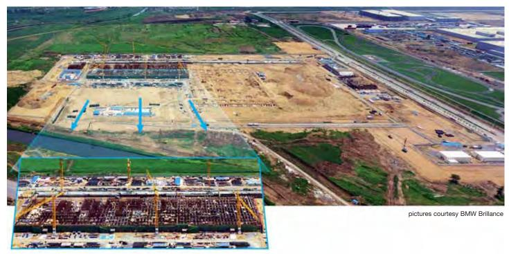
Aerial view of the site for the BMW Brilliance Automotive New Engine Plant in Shenyang, with the construction of the foundry currently under way (enlarged). The New Engine Plant is located next to BMW Brilliance Tiexi vehicle plant and high-speed testing circuit (on the right in the overall picture above)
