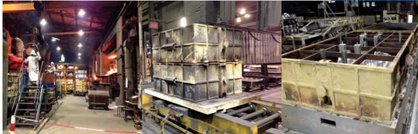
LOVINK TECHNOCAST, the foundry division of the corporation, requested GEMCO's assistance for an efficiency study. LOVINK TECHNOCAST recently set itself a few objectives: increase the number of pouring positions to optimize the tact time of its Lost Foam production line and reduce the cycle time for vacuum connections during and after casting.
