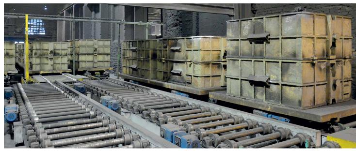
Figure 5: Automatic roller conveyor system for the shake-out station. Up to 25 t of mold boxes can be transported here
