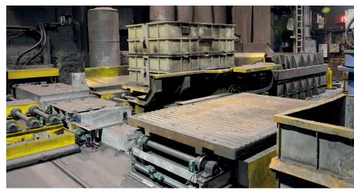
**Figure 6:** Shake-out station with a special lifting and tilting table from which the manipulator picks up molds and mold boxes
