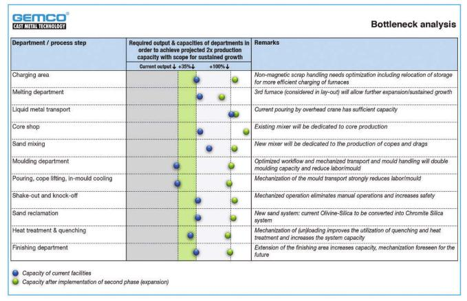
Figure 1: A capacity and bottleneck analysis was the first step towards doubling capacity at Nortrak in the USA.
