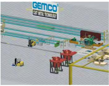
Horizontal moulding line with two induction furnaces
