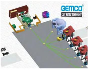
Possible set-up of four induction furnaces, one holder, and one pouring furnace
