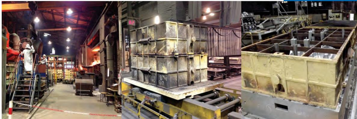
LOVINK TECHNOCAST, the foundry division of the corporation, requested GEMCO's assistance for an efficiency study. LOVINK TECHNOCAST recently set itself a few objectives: increase the number of pouring positions to optimize the tact time of its Lost Foam production line and reduce the cycle time for vacuum connections during and after casting.
