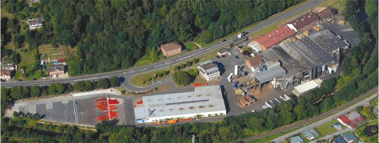
Aerial view of the Linde plant in Weilbach. With a workforce of 157, the plant produces around 180 counterweights for forklift trucks every day. The production volume is around 50,000 t per year (Photo: Linde)
