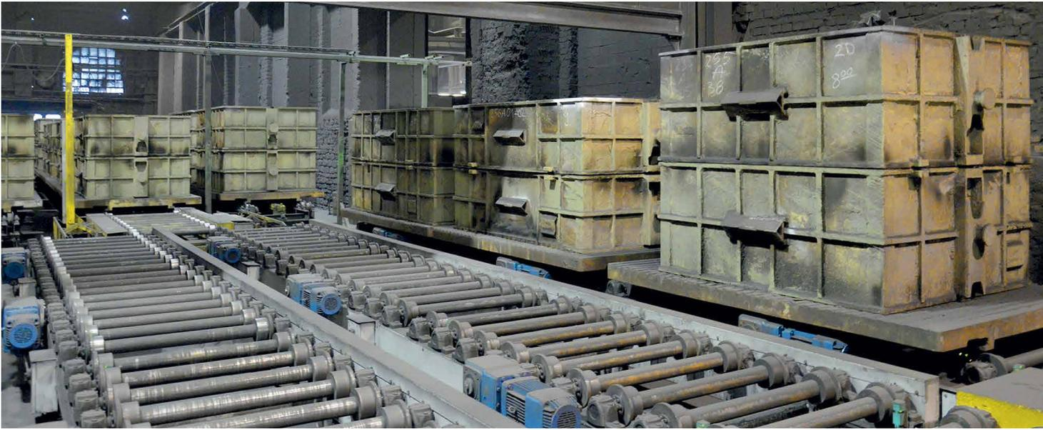
**Figure 5:** Automatic roller conveyor system for the shake-out station. Up to 25 t of mold boxes can be transported here
