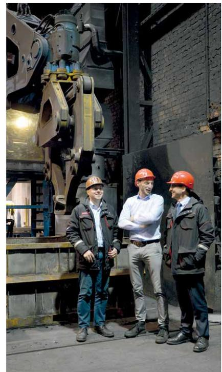
**Figure 4:** This specially developed manipulator separates molds and castings. In the foreground: Martin Severing (l.), Project Manager/Head of Engineering Counterweights, and Klemens Raub (r.), Plant Manager Linde Weilbach, with Maurits Brandt, Gemco Engineers
