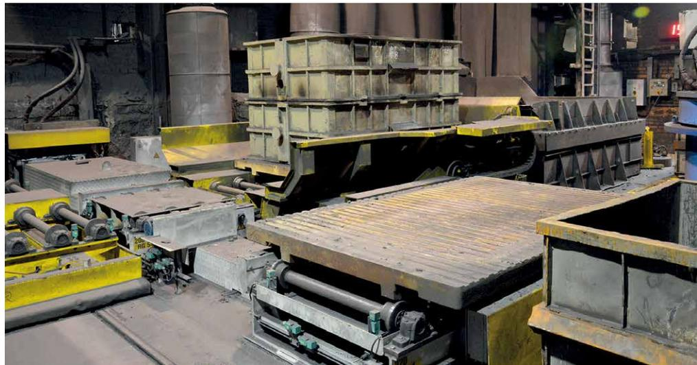
**Figure 6:** Shake-out station with a special lifting and tilting table from which the manipulator picks up molds and mold boxes
