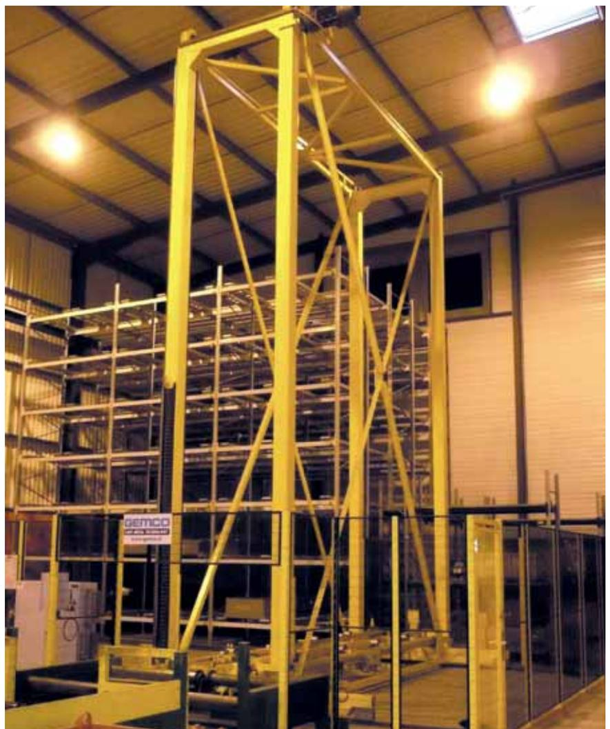
**Figure 2:** Pattern storage and manipulator
