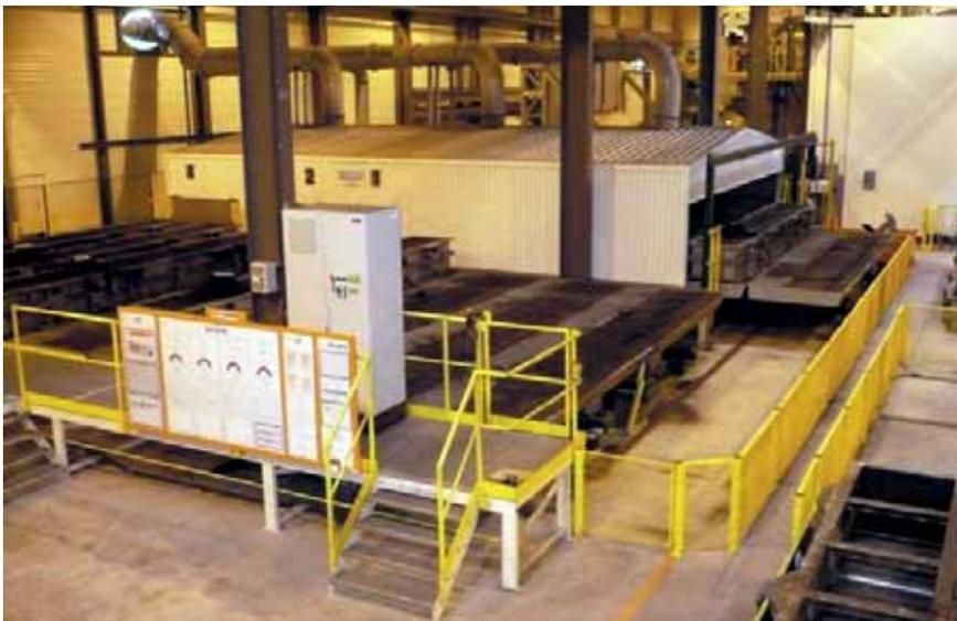
Figure 3: Pouring and cooling line, front row for pouring
