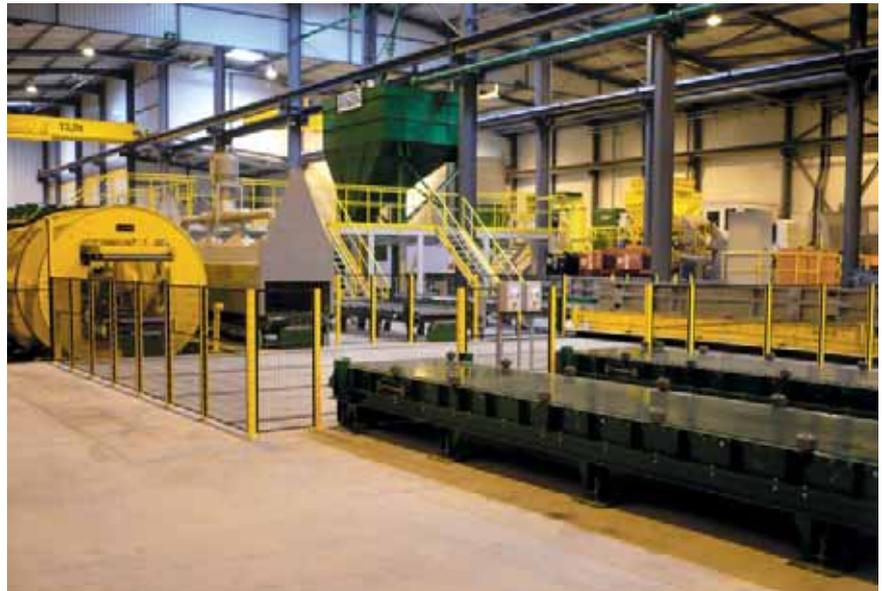
**Figure 1:** Moulding line: rollover closing unit and pouring cup setting in front coating drying, inspection and core setting and transfer car behind
