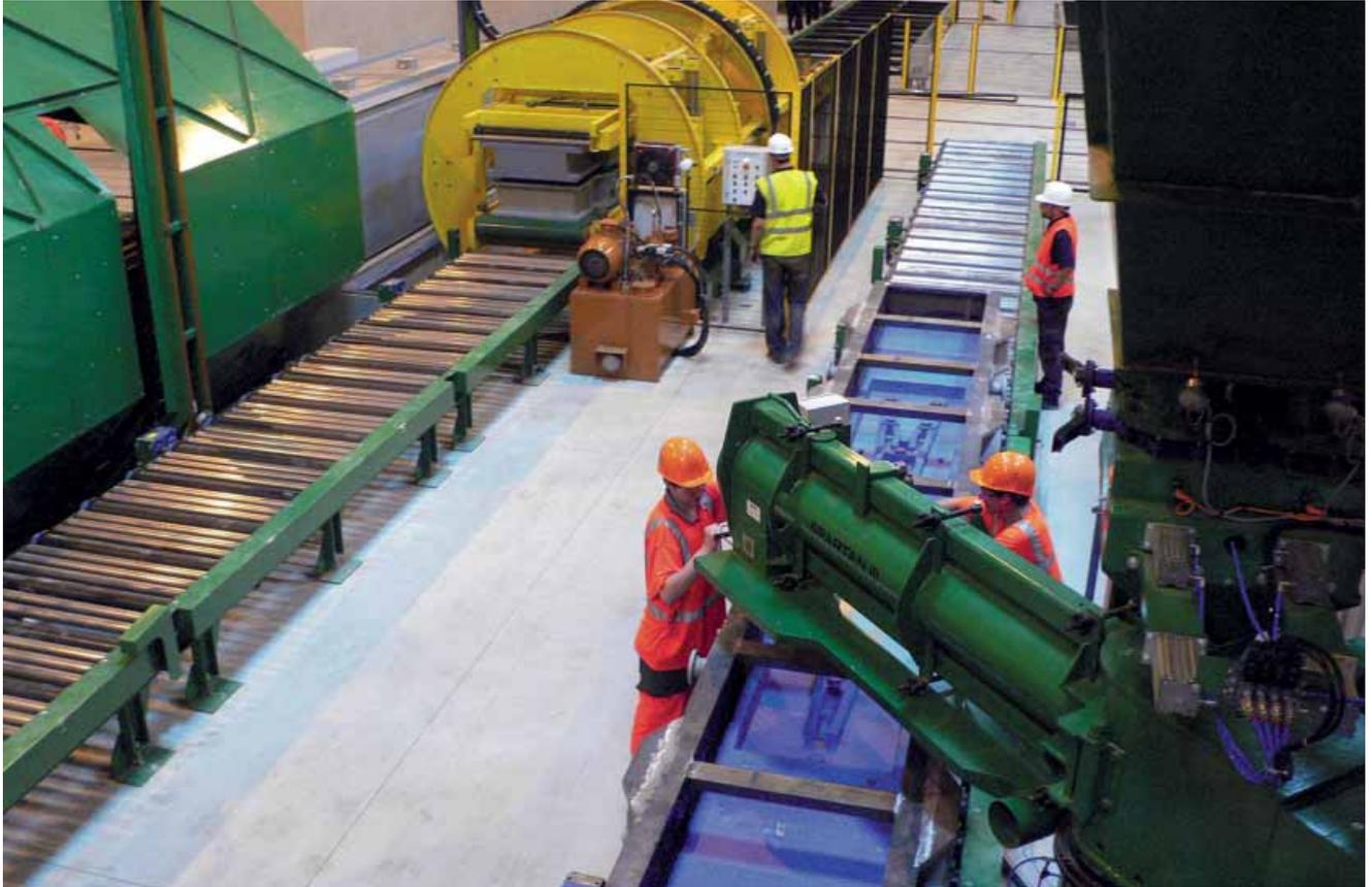
Moulding line: mixing and stripping (Photos: Gemco Engineers )
