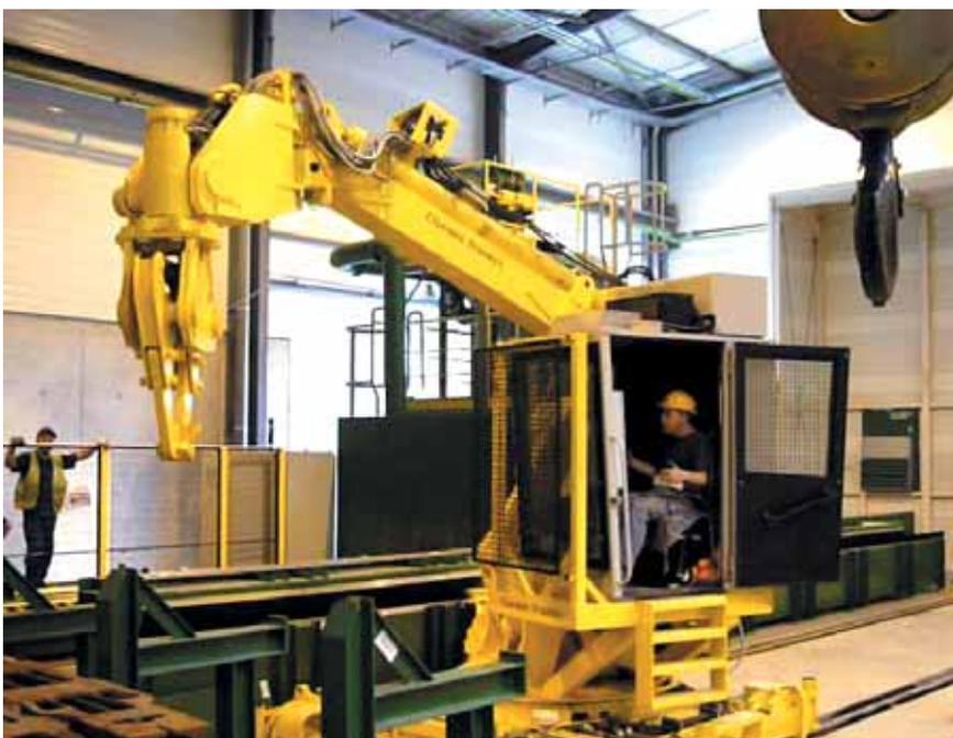
Figure 4: Heavy duty manipulator as operated after heat treatment and prior to grinding and welding booths
