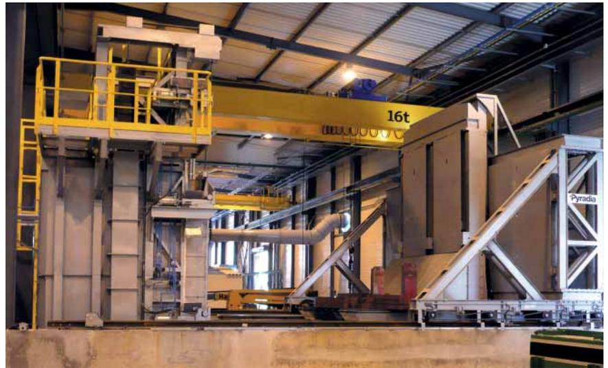
Figure 5: Heat treatment furnace with a 15 t automated manipulator for loading/unloading as well as quenching
