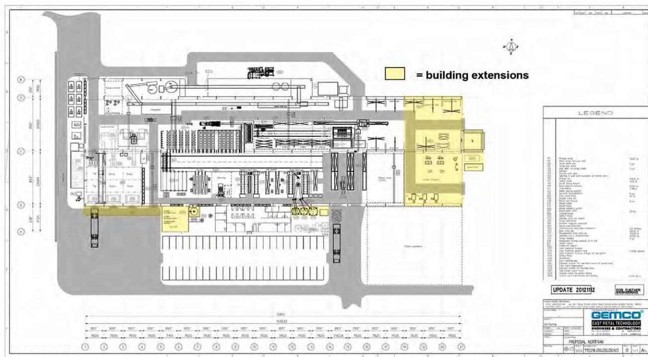
**Figure 3:** voestalpine Nortrak, Decatur, proposed layout in order to achieve projected capacity expansion (yellow= building extensions)
