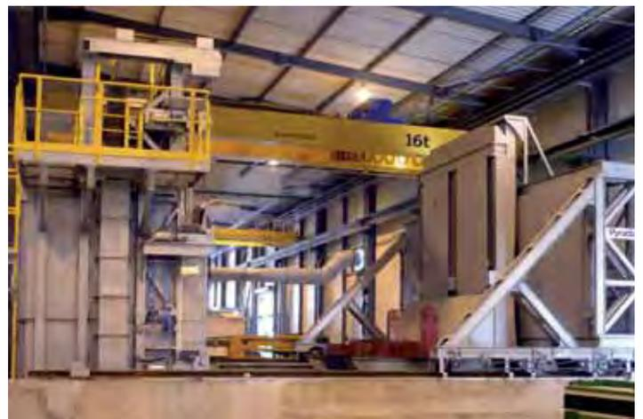
*Heat Treatment with automatic loading and quenching device*
