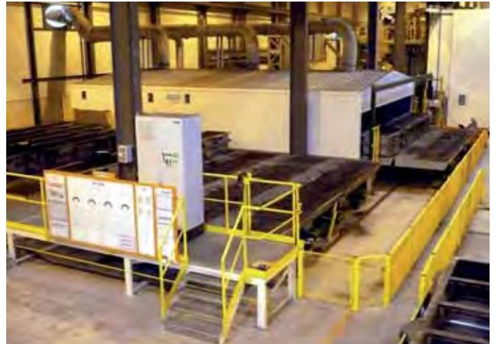
*Gemco-designed dedicated semi-automated pouring line and cooling tunnel*
