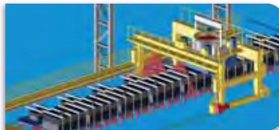
Cost, Safety & Efficiency: Automatic Pouring for 30 tons steel in bottom-pour ladles on no-bake moulding line
