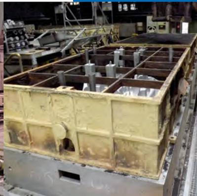
LOVINK TECHNOCAST, the foundry division of the corporation, requested GEMCO's assistance for an efficiency study. LOVINK TECHNOCAST recently set itself a few objectives: increase the number of pouring positions to optimize the tact time of its Lost Foam production line and reduce the cycle time for vacuum connections during and after casting.
